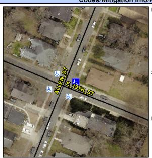
Street 1 Name **ALLEN ST** Stop Condition-Street 2 None Street 2 Name E 19TH ST Stop Condition-Street 1 StopSign Possible Solutions: Remove & Replace Curb Ramp With **Two New Directional Ramps or** Equivalent. Surveyor Notes: N/A PROW/ADA: Not Found, R304.5.3, R305.1.4, R305.2, R302.7.2
