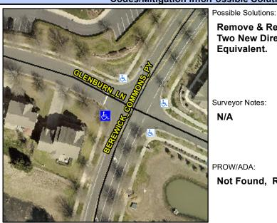
**BEREWICK COMMONS PY** Street 1 Name Stop Condition-Street 2 None Street 2 Name **GLENBURN LN** Stop Condition-Street 1 StopSign Remove & Replace Curb Ramp With **Two New Directional Ramps or** Equivalent.
