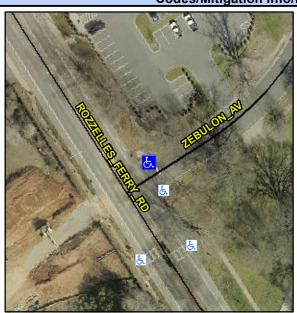
Street 1 Name **ROZZELLES FERRY RD** Stop Condition-Street 2 None Street 2 Name **ZEBULON AV** Stop Condition-Street 1 StopSign Possible Solutions: Remove & Replace Curb Ramp With **Two New Directional Ramps or** Equivalent. Surveyor Notes: N/A PROW/ADA: Not Found, R304.2.2, R304.5.3
