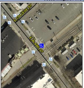
**E BLAND ST** Street 1 Name Stop Condition-Street 1 None Street 2 Name N/A Stop Condition-Street 2 N/A Possible Solutions: Remove & Replace Curb Ramp With **Two New Directional Ramps or** Equivalent. Surveyor Notes: N/A PROW/ADA: Not Found, R304.2.3
