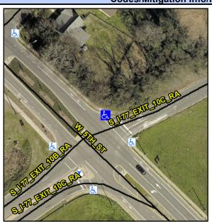
**S I-77 EXIT 10C RA** Street 1 Name Stop Condition-Street 1 StopSign N/A Street 2 Name Stop Condition-Street 2 N/A Possible Solutions: Remove & Replace Entire Ramp. Surveyor Notes: RT RP < 5% R304.3.2
