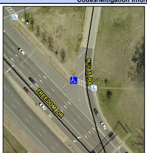
N I-85 RA Street 1 Name Stop Condition-Street 1 None Street 2 Name N/A Stop Condition-Street 2 N/A Possible Solutions: Remove & Replace Entire Ramp. Grind Gutter Lip. Surveyor Notes: N/A PROW/ADA: R304.5.3, R305.2, R302.7.2
