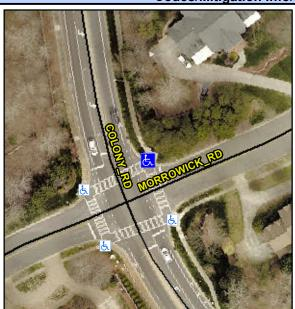
**COLONY RD** Street 1 Name Stop Condition-Street 2 Signal Street 2 Name MORROWICK RD Stop Condition-Street 1 Signal Possible Solutions: Remove & Replace Curb Ramp With Two New Dir Equivalent. Surveyor Notes: N/A
