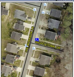
JOE MORRISON LN Street 1 Name Stop Condition-Street 2 None Street 2 Name SHUFFLETOWN DR Stop Condition-Street 1 StopSign Possible Solutions: Remove & Replace Curb Ramp With **Two New Directional Ramps or** Equivalent. Surveyor Notes: N/A PROW/ADA: Not Found, R304.5.1, R304.2.2
