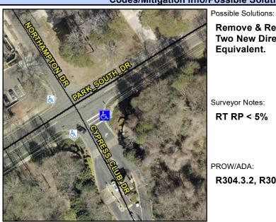
Stop Condition-Street 1 Street 2 Name Stop Condition-Street 2 **Remove & Replace Curb Ramp With** Two New Directional Ramps or Equivalent.
