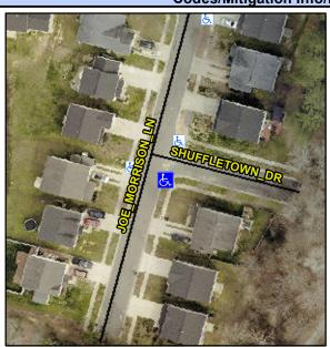
SHUFFLETOWN DR Street 1 Name Stop Condition-Street 2 StopSign **JOE MORRISON LN** Street 2 Name Stop Condition-Street 1 None Possible Solutions: Remove & Replace Curb Ramp With Two New Directional Ramps or Equivalent. Surveyor Notes: N/A PROW/ADA: R304.5.1, R304.5.3
