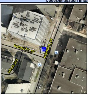
Street 1 Name Stop Condition-Street 2 Street 2 Name Stop Condition-Street 1 **DOGGETT ST** StopSign **HAWKINS ST** None Possible Solutions: Remove & Replace Curb Ramp With Two New Directional Ramps or Equivalent. Surveyor Notes: N/A PROW/ADA: R304.5.3
