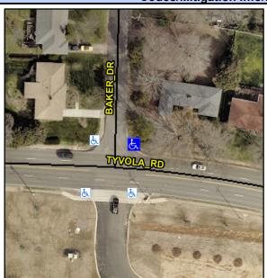
Street 1 Name StopSign **BAKER DR** Stop Condition-Street 1 Street 2 Name None Stop Condition-Street 2 **TYVOLA RD**  Possible Solutions: Remove & Replace Curb Ramp With Two New Directional Ramps or Equivalent. Surveyor Notes: N/A PROW/ADA: R304.5.1, R304.3.2
