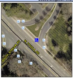
**ENTRANCE** Street 1 Name Stop Condition-Street 1 None Street 2 Name N/A Stop Condition-Street 2 N/A Possible Solutions: **Remove & Replace Curb Ramp With Two New Directional Ramps or** Equivalent. Surveyor Notes: **LOCATED ON ISLAND** PROW/ADA: R304.5.1, R304.5.3
