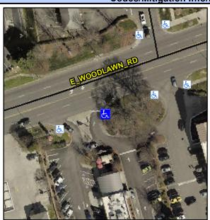
E WOODLAWN RD Street 1 Name Stop Condition-Street 2 None **ENTRANCE** Street 2 Name Stop Condition-Street 1 StopSign Possible Solutions: Compliance Description N/A Remove & Replace Curb Ramp With Two New Directional Ramps or Equivalent. Surveyor Notes: N/A PROW/ADA: Not Found, R304.5.3
