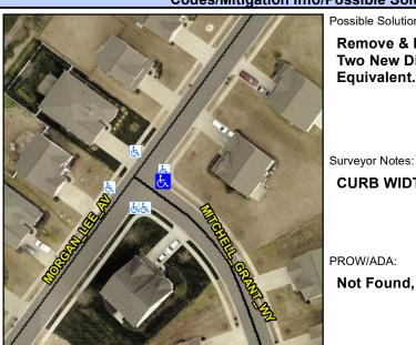
**MITCHELL GRANT WY** Street 1 Name Stop Condition-Street 1 StopSign Street 2 Name N/A Stop Condition-Street 2 N/A Possible Solutions: Remove & Replace Curb Ramp With **Two New Directional Ramps or** Equivalent.
