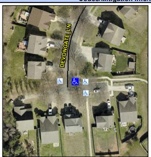
**DEVONGATE LN** Street 1 Name Stop Condition-Street 1 None N/A Street 2 Name Stop Condition-Street 2 N/A Possible Solutions: Remove & Replace Curb Ramp With Two New Directional Ramps or Equivalent. Surveyor Notes: N/A PROW/ADA: Not Found, R304.5.1
