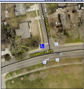
Street 1 Name Stop Condition-Street 2 Street 2 Name Stop Condition-Street 1 SHAMROCK DR None **FOXFORD PL** StopSign Possible Solutions: Remove & Replace Curb Ramp With Two New Directional Ramps or Equivalent. Surveyor Notes: N/A PROW/ADA: Not Found, R304.5.1
