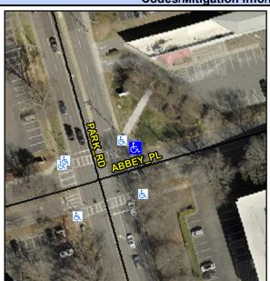
**ABBEY PL** Street 1 Name Stop Condition-Street 2 Signal Street 2 Name N/A Stop Condition-Street 1 N/A Possible Solutions: Remove & Replace Entire Ramp. Restripe Crosswalk. Surveyor Notes: N/A PROW/ADA: R304.2.2
