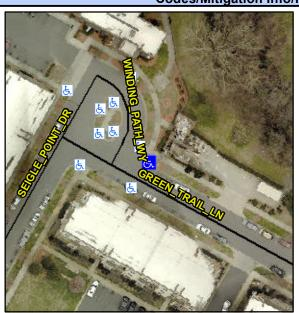
**GREEN TRAIL LN** Street 1 Name Stop Condition-Street 2 None Street 2 Name N/A Stop Condition-Street 1 N/A Possible Solutions: Remove & Replace Entire Ramp. Remove & Replace Gutter. Surveyor Notes: N/A PROW/ADA: Not Found, R304.5.3, R304.2.2-Perp, R304.3.2-Para
