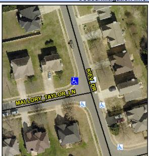
**MALLORY TAYLOR LN** Street 1 Name Stop Condition-Street 2 StopSign **KIEV DR** Street 2 Name Stop Condition-Street 1 None Possible Solutions: Remove & Replace Curb Ramp With Two New Directional Ramps or Equivalent. Surveyor Notes: N/A PROW/ADA: Not Found, R304.5.1
