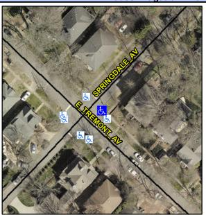
**SPRINGDALE AV** Street 1 Name Stop Condition-Street 1 StopSign N/A Street 2 Name Stop Condition-Street 2 N/A Possible Solutions: Remove & Replace Entire Ramp. Surveyor Notes: N/A PROW/ADA: R304.5.1, R304.5.3
