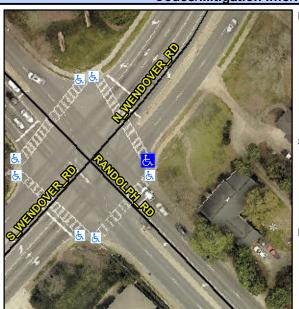
N WENDOVER RD Street 1 Name Stop Condition-Street 2 Signal Street 2 Name N/A Stop Condition-Street 1 N/A Possible Solutions: Remove & Replace Entire Ramp. Surveyor Notes: N/A PROW/ADA: Not Found, R304.5.1, R304.5.3
