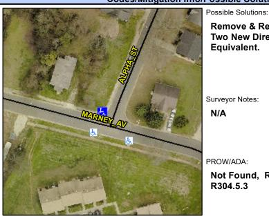
**MARNEY AV** Street 1 Name Stop Condition-Street 2 Street 2 Name **ALPHA ST** Stop Condition-Street 1 StopSign **Remove & Replace Curb Ramp With** Two New Directional Ramps or Equivalent.
