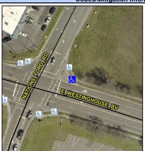
**E WESTINGHOUSE BV** Street 1 Name Stop Condition-Street 2 Signal Street 2 Name N/A Stop Condition-Street 1 N/A Possible Solutions: Remove & Replace Entire Ramp. Restripe Crosswalk. Surveyor Notes: N/A PROW/ADA: Not Found, R304.5.1, R304.5.3
