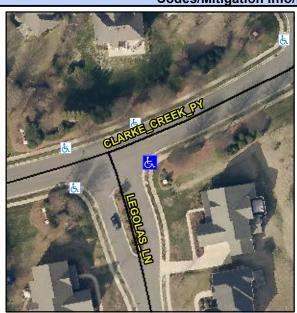
**CLARKE CREEK PY** Street 1 Name Stop Condition-Street 2 **LEGOLAS LN** Street 2 Name Stop Condition-Street 1 StopSign Possible Solutions: Remove & Replace Curb Ramp With Two New Directional Ramps or Equivalent. Surveyor Notes: N/A PROW/ADA: R304.5.1
