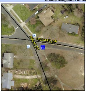
Street 1 Name Stop Condition-Street 1 Street 2 Name Stop Condition-Street 2 **HILLIARD DR** None **AIRLIE ST** StopSign Possible Solutions: **Remove & Replace Curb Ramp With** Two New Directional Ramps or Equivalent. Surveyor Notes: N/A PROW/ADA: R304.5.1
