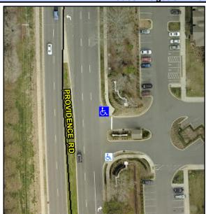
Street 1 Name None Stop Condition-Street 1 PROVIDENCE RD Street 2 Name StopSign Stop Condition-Street 2 N/A Possible Solutions: Remove & Replace Curb Ramp With Two New Directional Ramps or Equivalent. Surveyor Notes: RT RP < 5% PROW/ADA Not Found, R304.5.1, R304.2.2, R304.5.3, R304.3.2
