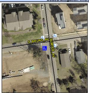
Street 1 Name SUMTER AV Stop Condition-Street 2 StopSign **S BRUNS AV** Street 2 Name Stop Condition-Street 1 StopSign Possible Solutions: Compliance Description N/A Remove & Replace Curb Ramp With Two New Directional Ramps or No Equivalent. N/A N/A N/A N/A Surveyor Notes: N/A N/A N/A N/A N/A N/A PROW/ADA: N/A R304.5.1, R304.2.2 N/A N/A N/A N/A
