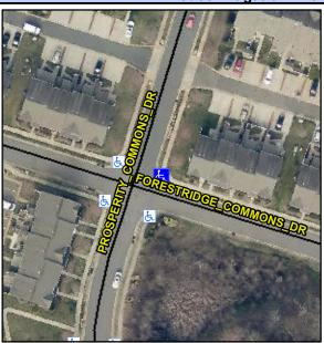
Stop Condition-Street 2 Street 2 Name Stop Condition-Street 1 Possible Solutions: Remove & Replace Curb Ramp With Two New Directional Ramps or Equivalent.
