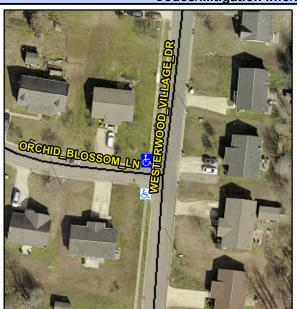
**ORCHID BLOSSOM LN** Street 1 Name Stop Condition-Street 1 StopSign Street 2 Name N/A Stop Condition-Street 2 N/A Possible Solutions: Remove & Replace Curb Ramp With Two New Directional Ramps or Equivalent. Surveyor Notes: N/A PROW/ADA: R304.5.1, R304.5.3
