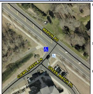
**CLEMS CREEK LN** Street 1 Name Stop Condition-Street 1 StopSign N/A Street 2 Name Stop Condition-Street 2 N/A Possible Solutions: Remove & Replace Entire Ramp. Surveyor Notes: N/A PROW/ADA: R304.5.3
