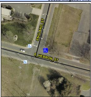
**ENGLAND ST** Street 1 Name Stop Condition-Street 2 StopSign Street 2 Name **E HEBRON ST** Stop Condition-Street 1 None Possible Solutions: Remove & Replace Curb Ramp With **Two New Directional Ramps or** Equivalent. Surveyor Notes: N/A PROW/ADA: Not Found, R304.5.1, R304.5.3
