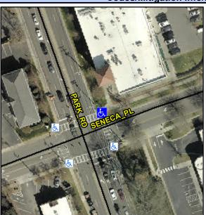
**PARK RD** Street 1 Name Stop Condition-Street 2 Signal Street 2 Name **SENECA PL** Stop Condition-Street 1 Signal Possible Solutions: Remove & Replace Curb Ramp With **Two New Directional Ramps or** Equivalent. Surveyor Notes: N/A PROW/ADA: Not Found, R304.2.2
