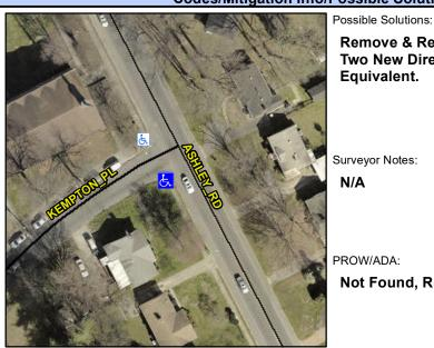
**KEMPTON PL** Street 1 Name Stop Condition-Street 1 StopSign Street 2 Name N/A Stop Condition-Street 2 N/A **Remove & Replace Curb Ramp With Two New Directional Ramps or** Equivalent.
