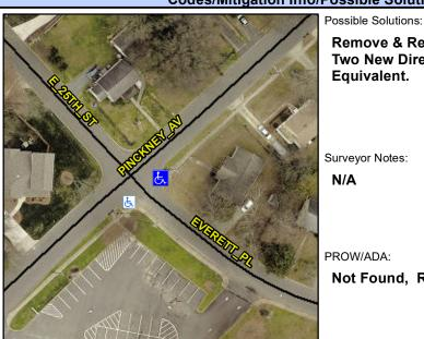
**EVERETT PL** Street 1 Name Stop Condition-Street 1 StopSign Street 2 Name N/A Stop Condition-Street 2 N/A Remove & Replace Curb Ramp With Two New Directional Ramps or Equivalent.
