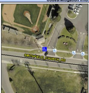
**ENTRANCE** Street 1 Name Stop Condition-Street 1 StopSign Street 2 Name N/A Stop Condition-Street 2 N/A Possible Solutions: Compliance Description Remove & Replace Curb Ramp With N/A Two New Directional Ramps or No Equivalent. Surveyor Notes: N/A PROW/ADA: Not Found, R304.5.1
