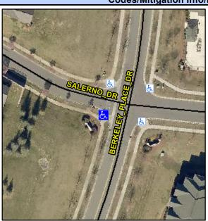
BERKELEY PLACE DR Street 1 Name Stop Condition-Street 2 None **SALERNO DR** Street 2 Name Stop Condition-Street 1 StopSign Possible Solutions: Remove & Replace Curb Ramp With Two New Directional Ramps or Equivalent. Surveyor Notes: N/A PROW/ADA: R304.2.2
