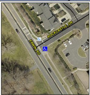
Street 1 Name Stop Condition-Street 2 Street 2 Name Stop Condition-Street 1 **ROCKCASTLE DR** StopSign **ERWIN RD** None Possible Solutions: Remove & Replace Curb Ramp With **Two New Directional Ramps or** Equivalent. Surveyor Notes: N/A PROW/ADA: Not Found, R304.5.1, R304.5.3
