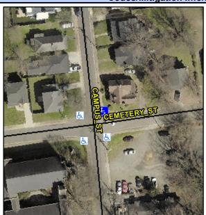
**CAMPUS ST** Street 1 Name Stop Condition-Street 2 None Street 2 Name **CEMETERY ST** Stop Condition-Street 1 StopSign Possible Solutions: Remove & Replace Curb Ramp With **Two New Directional Ramps or** Equivalent. Surveyor Notes: N/A PROW/ADA: Not Found, R304.5.1, R304.2.2, R304.5.3
