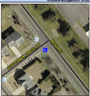
MOSS RD Street 1 Name Stop Condition-Street 2 None SCOTTSMAN TRACE DR Street 2 Name Stop Condition-Street 1 StopSign Possible Solutions: Remove & Replace Curb Ramp With Two New Directional Ramps or Equivalent. Surveyor Notes: N/A PROW/ADA: R304.2.2
