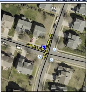
**GAILES DR** Street 1 Name Stop Condition-Street 2 None **SEDGEBURN DR** Street 2 Name Stop Condition-Street 1 StopSign Possible Solutions: Remove & Replace Curb Ramp With Two New Directional Ramps or Equivalent. Surveyor Notes: N/A PROW/ADA: R304.5.1
