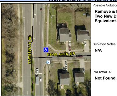
**NEVIN GLEN DR** Street 1 Name Stop Condition-Street 1 StopSign Street 2 Name N/A Stop Condition-Street 2 N/A Possible Solutions: **Remove & Replace Curb Ramp With Two New Directional Ramps or** Equivalent.
