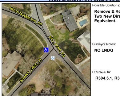
Street 1 Name Stop Condition-Street 1 Street 2 Name Stop Condition-Street 2 **JOHNNY CAKE LN** StopSign MILL POND RD Remove & Replace Curb Ramp With Two New Directional Ramps or Equivalent.
