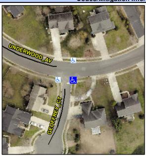
Street 1 Name Stop Condition-Street 2 Street 2 Name Stop Condition-Street 1 **UNDERWOOD AV** None **GEOFFREY CT** StopSign Possible Solutions: **Remove & Replace Curb Ramp With Two New Directional Ramps or** Equivalent. Surveyor Notes: N/A PROW/ADA: Not Found, R304.5.1, R304.5.3
