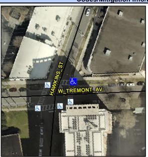
**HAWKINS ST** Street 1 Name Stop Condition-Street 2 StopSign Street 2 Name W TREMONT ST Stop Condition-Street 1 StopSign Possible Solutions: Remove & Replace Curb Ramp With **Two New Directional Ramps or** Equivalent. Surveyor Notes: N/A PROW/ADA: R304.2.2, R304.5.3
