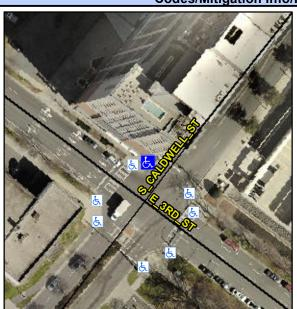
S CALDWELL ST Street 1 Name Signal Stop Condition-Street 2 Street 2 Name N/A Stop Condition-Street 1 N/A Possible Solutions: Remove & Replace Entire Ramp. Surveyor Notes: N/A PROW/ADA: R304.2.2
