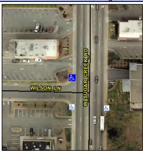
WILSON LN Street 1 Name Stop Condition-Street 1 StopSign Street 2 Name W SUGAR CREEK RD Stop Condition-Street 2 None Possible Solutions: Remove & Replace Curb Ramp With Two New Directional Ramps or Equivalent. Surveyor Notes: N/A PROW/ADA: R304.3.2
