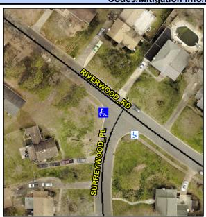
Street 1 Name Stop Condition-Street 1 Street 2 Name Stop Condition-Street 2 SURREYWOOD PL StopSign **RIVERWOOD RD** None Possible Solutions: **Remove & Replace Curb Ramp With** Two New Directional Ramps or Equivalent.
