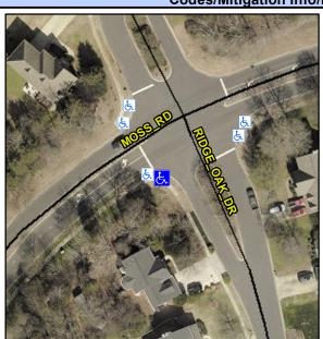
**RIDGE OAK DR** Street 1 Name Stop Condition-Street 1 StopSign Street 2 Name N/A Stop Condition-Street 2 N/A **Remove & Replace Curb Ramp With Two New Directional Ramps or** Equivalent.
