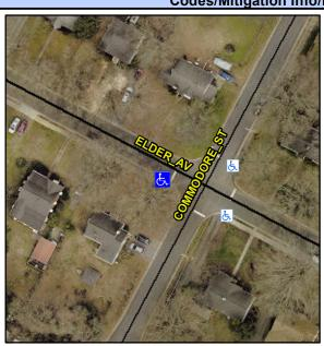
**ELDER AV** Street 1 Name Stop Condition-Street 1 None Street 2 Name N/A Stop Condition-Street 2 N/A Remove & Replace Curb Ramp With **Two New Directional Ramps or** Equivalent.
